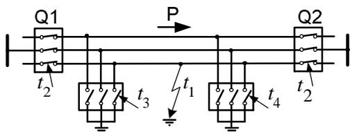
Fig. 11. Transmission line with high speed grounding switches.
